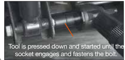
Holding socket fits over the bolt and prevents it rotating.
