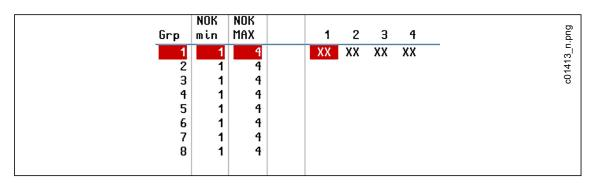
Abb. 5-13: Example 2 has one error handling group with all four tools assigned
