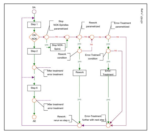
Abb. 5-19: Flowchart for touch-up and error handling
