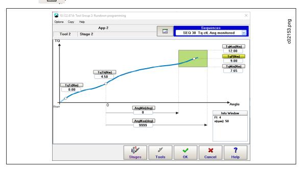
Abb. 5-5: The graphical view of the Rundown programming window
