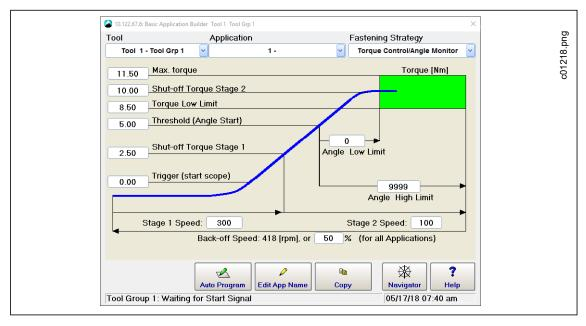
Abb. 3-1: Basic Application Builder window with the Torque Control/Angle Monitor fastening strategy selected
