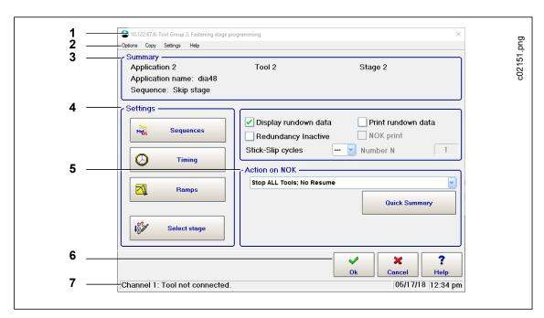
Abb. 5-3: The Fastening stage programming window set for programming Stage 2 of Tool 2 in Tool Group 2 for Application 2
