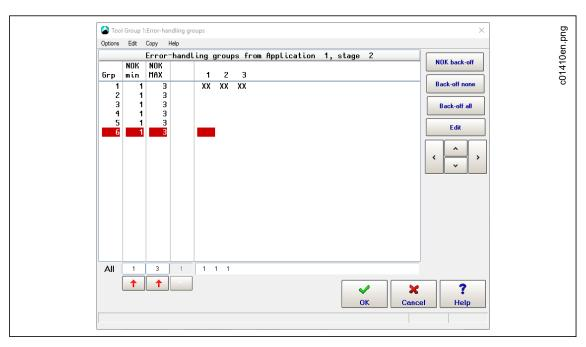
Abb. 5-9: Error Handling groups dialog with six error handling group (represented by table rows) and three tools (represented by table columns no. 1-3)
