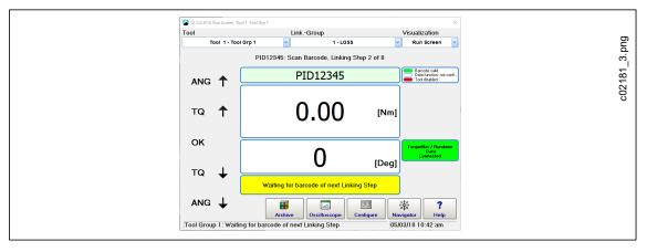
Fig. 8-6: Run screen displays Waiting for barcode of next Linking Step message
