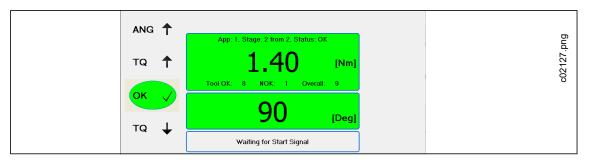
Abb. 4-2: The green background indicates that Tool 1 of Tool Group 1 has run successfully in Application 1
