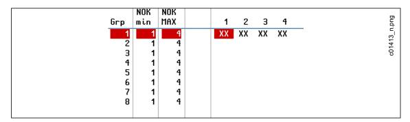
Abb. 5-16: Example 4 has one error handling group with all four tools assigned
