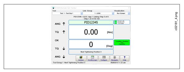
Fig. 8-7: Run screen displays Next Tightening Position 3 message
