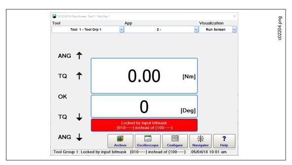
Abb. 5-27: Messages in the Status bar and in the Run Screen's Status field indicate that the Inputs defined for Application 2 in the Input / Output bitmask ('1' for Input 1, '0' for Input 2, '0' for Input 3, and Inputs 4 to 8 not defined) are not matched ('0' for Input 1, '1' for Input 2, '0' for Input 3). The tool is locked.
