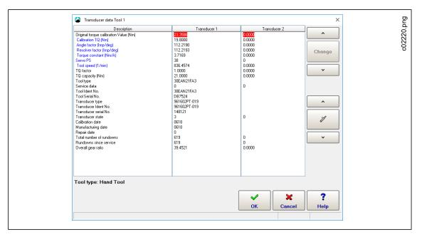
Abb. 7-2: The Transducer data screen for Tool 1
