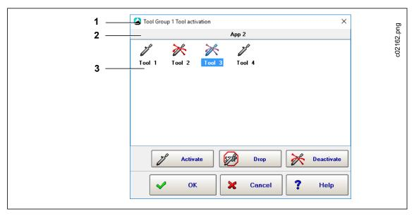
Abb. 5-1: The Tool activation dialog with the tools of Tool Group 1 used for Application 1. Tools 1 and 4 are activated, Tools 2 and 3 are deactivated. Tool 3 is currently selected.
