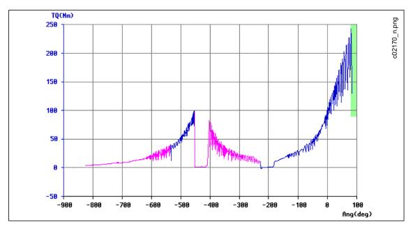
Abb. 5-6: Torque graph showing many stick-slip flanks
