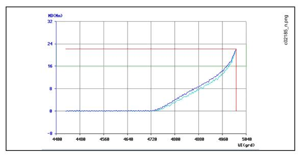
Fig. 4-5: The Torque graph view with the redundancy curve displayed in light blue color
