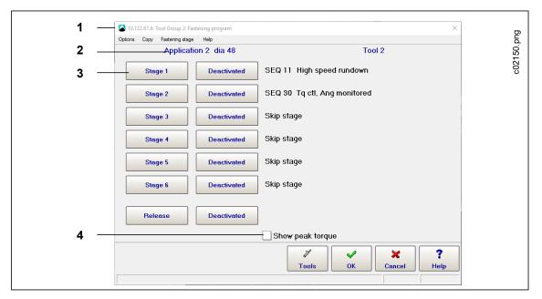
Abb. 5-2: The Fastening program window set for programming the stages of Tool 2 in Tool Group 2 for Application 2
